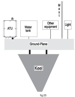
All equipment, mast, and light should be connected to this ground-plane seperately - not in the "daisey chain" manner.
