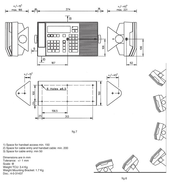
Transceiver Control Unit with Mounting Bracket.
