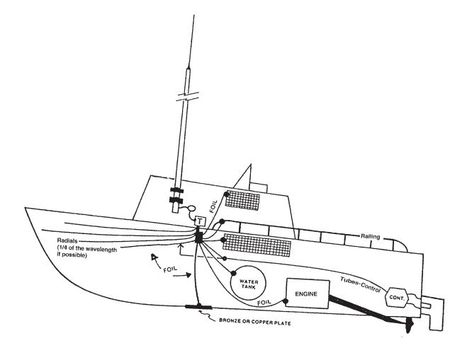
fig.26 Non-Metal Hull Grounding
