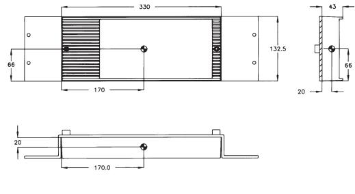
Dimensions are in mm Weight: DCU 1.2 Kg Tolerance: +/- 1 mm Centre of Gravity
