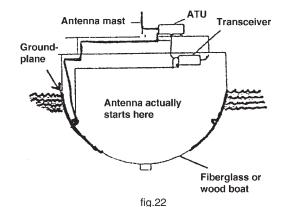
Wrong ATU placement on a fiberglass or wooden boat. All boxes, including the operator, is part of the antenna.
