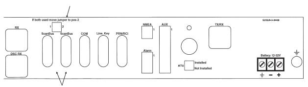
The ScanBus termination jumper must be set to pos. 1 if just one of the ScanBus connectors are used - and to pos. 2 if both ScanBus are used.
