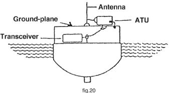
Put the ATU at the antenna groundplane on a metal boat
