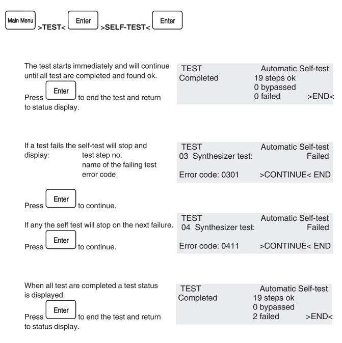
The error code consists of step number (2 digits), indication of previous faults (1 digit: 0=no, 1=yes) and failure type (1 digit).
