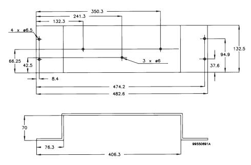
Dimensions are in mm Tolerance: +/- 0.2 mm
