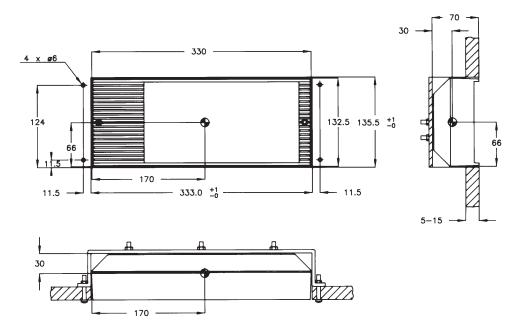
Dimensions are in mm Weight: DCU 1.2 Kg Tolerance: +/- 1 mm Weight: Mounting Bracket 0.7 Kg Centre of Gravity
