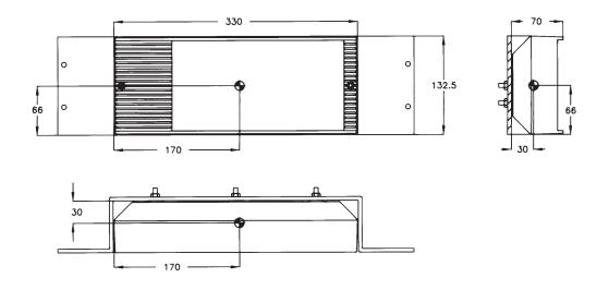
Dimensions are in mm Weight: DCU 1.2 Kg Tolerance: +/- 1 mm Weight: Mounting Bracket 0.7 Kg Centre of Gravity
