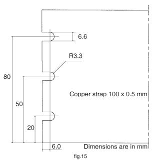
Should it be necessary to break the copper strap, for example to pass through a deck, two or three 1/2" or M12 bolts should be used for this feed through.
