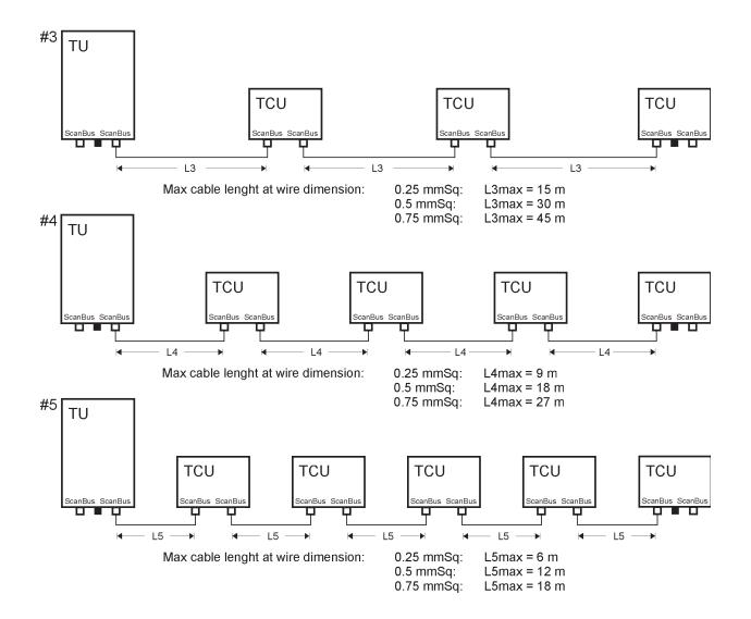
Installation examples and recommanded cable specification including the DSC option. Cable type: 2 x 5 screened multiwire ScanBus termination jumper:
