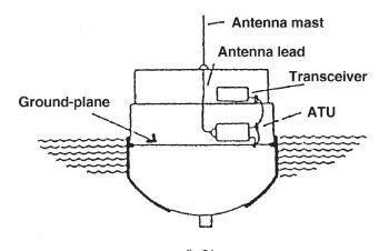
fig.21 Put the ATU at the antenna groundplane on a fiberglass or wooden boat
