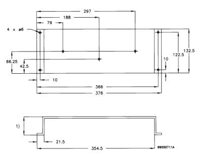
1) Customize to Bulkhead thickness. Dimensions are in mm Tolerance: +/- 0.2 mm
