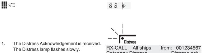
The display shows which station has acknowled the Distress Alert.
