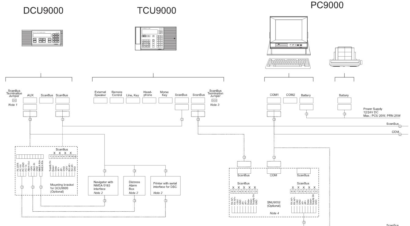
Note 1: If both ScanBus connectors are used remove jumper.
