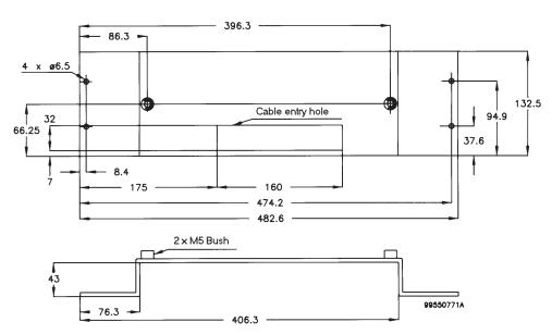
Dimensions are in mm Tolerance: +/- 0.2 mm CABLE CONNECTIONS FOR DCU WITHOUT MOUNTING BRACKET Fig.13
