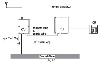
The coaxial- and multicables may be connected to equipment with a different ground potential. This will cause a loop-current.
