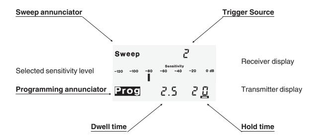
**Sweep annunciator :** Will be on during the programming and will flash during a frequency Sweep.
