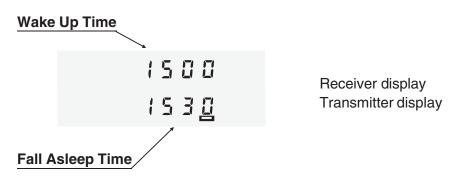
Wake Up Time: At this time the Sleep Program will switch on the transceiver.
