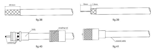
Remember to fit the rubber gasket on the coaxial cable before soldering.
